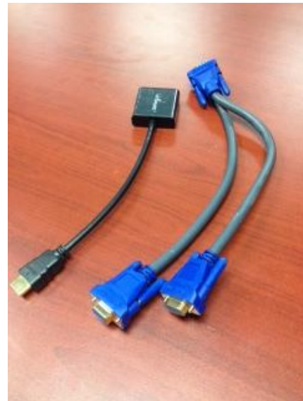
VGA Cable (right) HDMI to VGA adapter (left)
